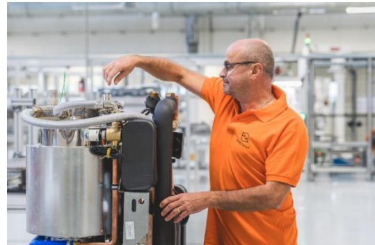
Assembly of the BOOSTHEAT.20's thermodynamic module
